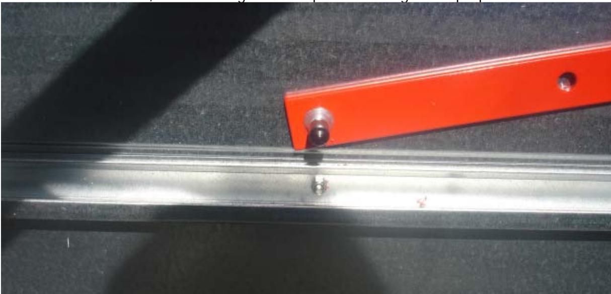
**14. The installation is complete once the threadlock has hardened (where applicable).** Threadlock continues to harden for 24 hours. The Shackle can be used immediately. Well done ☺
